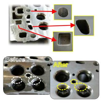
Valve sheet is harden material which is inserted in aluminum alloy body at intersection on the face where burr generated due to machining is successfully removed
