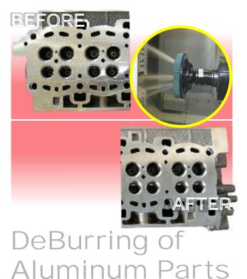
In the complete process of DeBurring, we recommend to use biggest size or at least one size bigger brush of that of the cutter size. We have brush sizes ranging from Ø 60, Ø 80, Ø 100, Ø 115, Ø 125, Ø 150, Ø 165, Ø 180, Ø 200, Ø 225, Ø250, Ø 296 and above.
