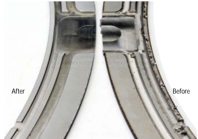
Hydro-generator S. S. Distributor Ring 2.5mm thick, ø 500mm grooved milled to depth 1.5mm, O.D. & I.D. laser cut duly DeBurred on VMC.
